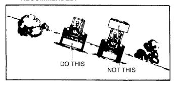
When transporting the load, keep the bucket as low as possible to avoid tipping in case a wheel drops into a rut.
